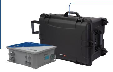
**Rugged Monitoring Ultra High Frequency** Partial Discharge (PD) monitoring solution is a platform that enables HV asset owners to monitor PD due to insulation defects 24/7. System can also be used to perform offline PD measurement during HV AC testing. Compact size and rugged enclosure of monitor makes it easy to get installed and get started.
